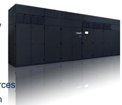
The UB-V Series UPS is Piller's latest generation of UPS. A completely new electronics platform affords even higher Reliability through advanced self-diagnostics and a revised internal architecture employing a unique real-time Ethernet communication protocol known as PillerLINK™. A patented ring topology provides redundancy between electronic boards powered by redundant power supplies that are fed from redundant sources.
